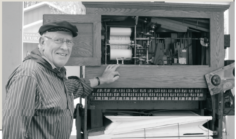
Gerry Koolen of Port Franks explains the inner workings of the fully-mobile Wurlitzer model 147 military band organ. The instrument, once steam-driven, is now powered by a portable electrical generator.
