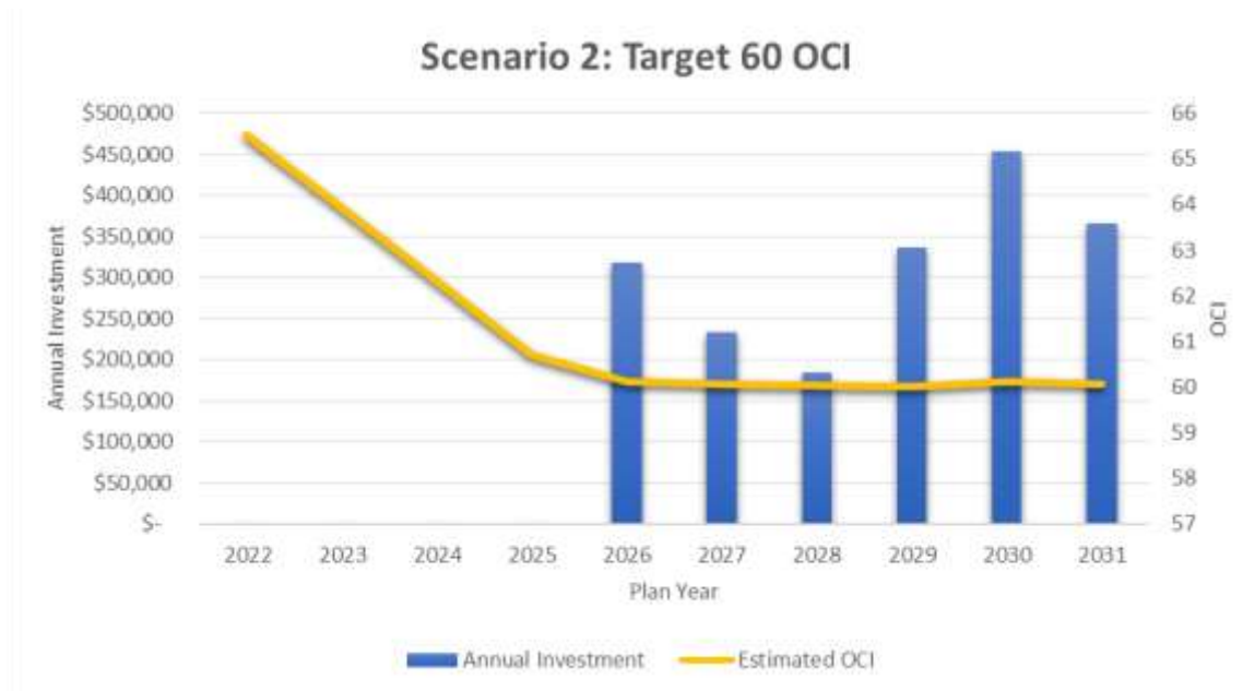
Figure 7-7: Scenario 2: Target 60 OCI - Storm Culvert Network Analysis
